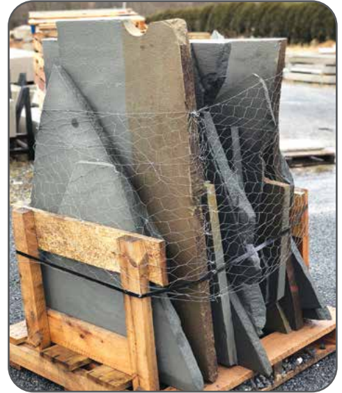
Sawn Bluestone 1.5" (Gauged) Sawn Thermal Finish (smoother finish)
